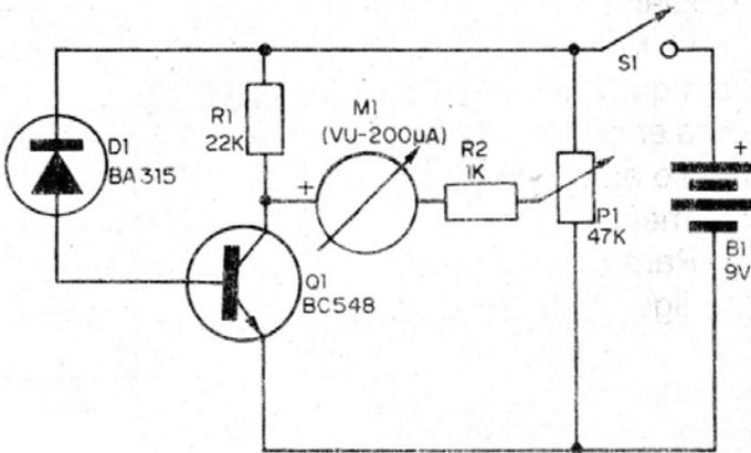
FIGURE 2 – SCHEMTAIC DIAGRAM OF THE DETECTOR
