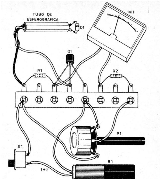
FIGURE 2 – MOUNTING USING A TERMINAL STRIP
