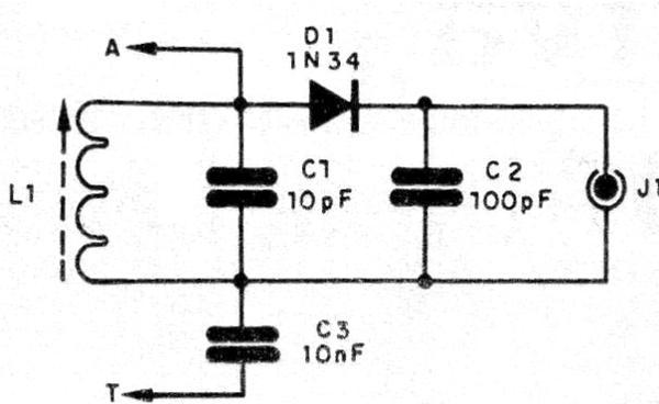
FIGURE 1 – SCHEMATIC DIAGRAM OF THE RADIO
